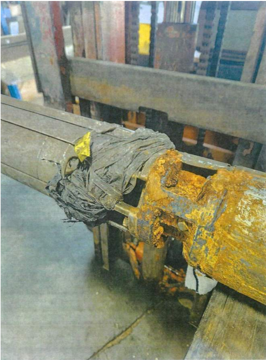
Plastic bags entwined in pump impeller.
